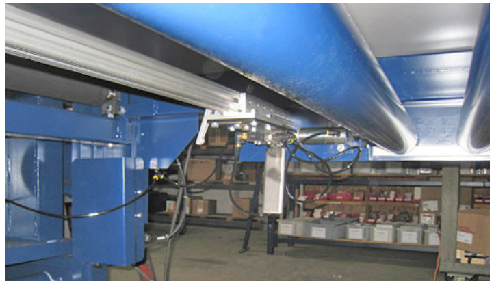
Automatic belt tracking features a new, heavy-duty design that is less susceptible to moisture and pressure fluctuations in compressed air. Easy to use and prolongs belt life.
