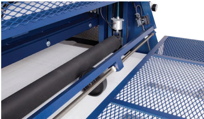
Detail of adjustable rubber-coated pinch roller and sheet sensor wheel.
