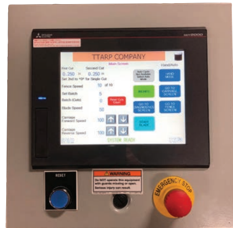
Touch-screen interface (mounts on a moveable console) enables easy set-up, easy adjustments, and easy recipe saving.
